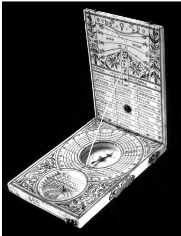
FIG. 13. Length of the day by season, gazetteer, string-gnomon horizontal dial for six latitudes, and scaphe for Nuremberg and Italian hours. Ivory diptych by Leonhart Miller, Nuremberg, 1613. Collection of Historical Scientific Instruments, Harvard University, 7459.
