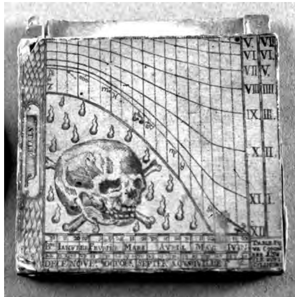
FIG. 18. Altitude dial with an hour scale dripping blood and a skull. Paper, French, late seventeenth century. Collection of Historical Scientific Instruments, Harvard University, 7173.
